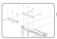
No. 2 M8x50 screws No. 2 M8 nuts 2 washers 8.4x17x1.5 No. 6 M4.8x25 screws
