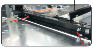
No. 2 M6x20 screws No. 2 M6 nuts 2 washer 6.5x14x1.5
